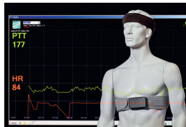
Devices (headband and chest band) for measuring a patient's vital parameters with a screen display of the data being monitored in the background. Photo: Fraunhofer IPMS
