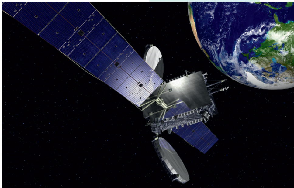
Geostationary satellites orbit the Earth once a day along the equator. Photo: SES
