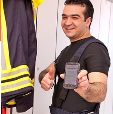
ECG and respiratory rate of firefighters are detected by the t-shirt and transmitted in real time via radio, for example, to a smartphone or directly into the command center. Photo: Fraunhofer IIS
